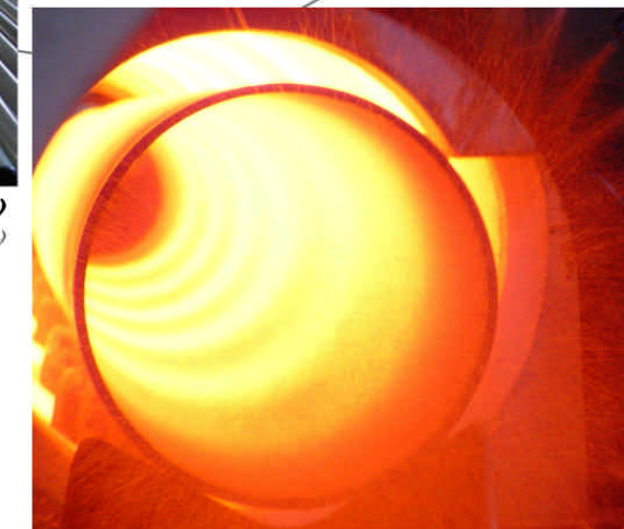
大径管用連続熱処理炉 Continuous Annealing Furnace
